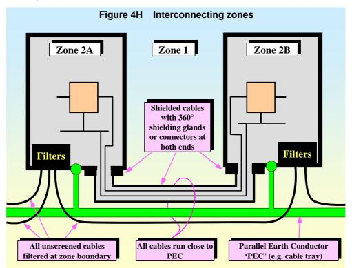
All screened cables that enter or leave shielded zones must have their screens terminated by  $360^{\circ}$  electrical contacts in shielding glands (or connectors) at the enclosure walls. Where the zone is simply defined by a MESH-CBN, high-frequencies will not be shielded against (depending on mesh size) but still the screened cables must be bonded at the zone boundary, for example by using a saddleclamp to bond them at the filter bonding plate shown in Figure 4E above.
