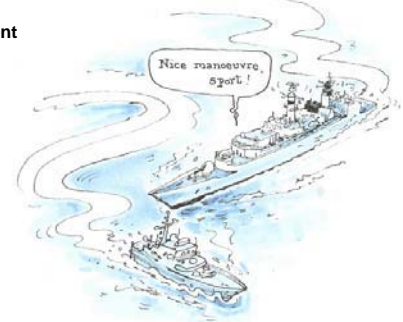
The steering of an Australian Navy minesweeper was affected by the radar of a nearby ship, nearly causing a collision
