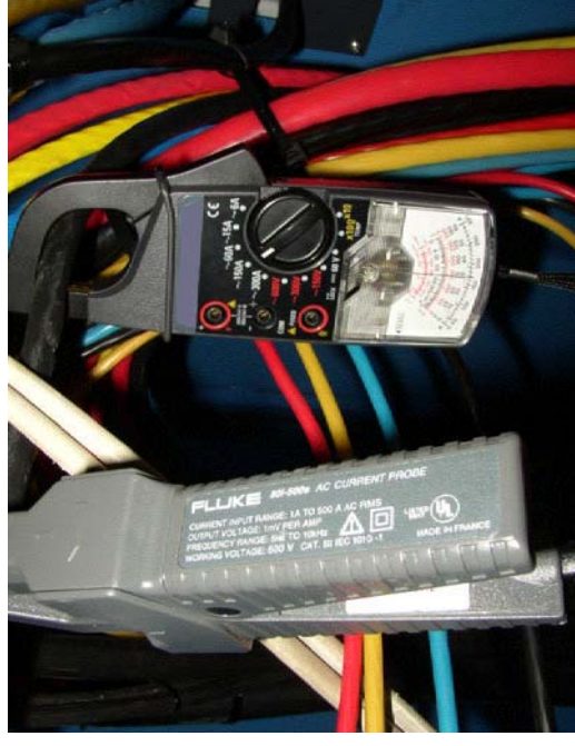
Figure 13 Comparing a True-RMS ammeter with an ordinary electricians clamp-on ammeter
