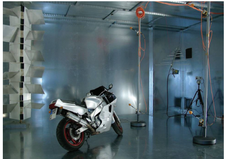
Figure 5: Example of a reverberation or stirred-mode chamber: The (large) Reverberation Chamber at Otto-von-Guericke-University Magdeburg, Germany
