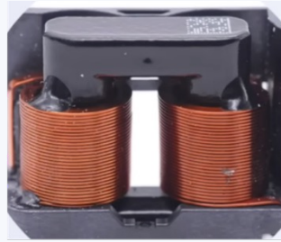
Flat-wire winding on a sectional wound CMC
