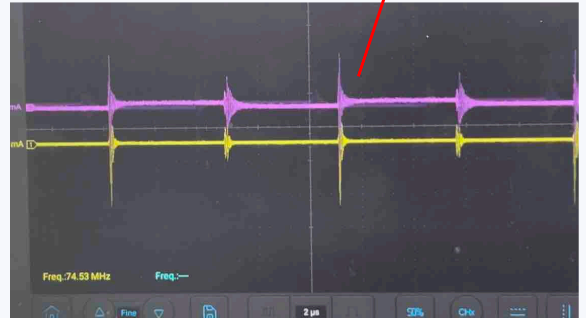
Forward common mode current and return current
