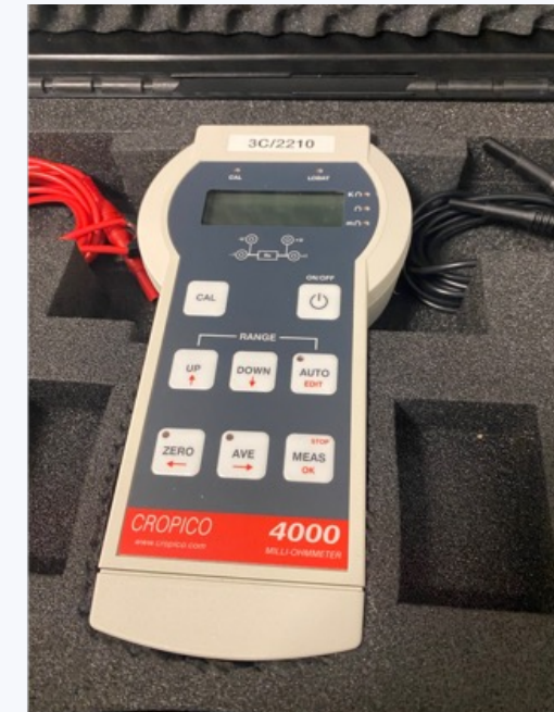
A popular milli-ohmmeter used for checking the continuity of the ground plane and LISN connections
