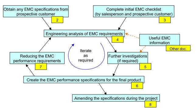
To decide what EMC performance is needed for the final product, it is commonplace in some industries for each project to begin with a full EMC site survey in an attempt to fully characterise the electromagnetic environment that it will be expected to operate in. But an EMC site survey can only measure an existing site, and planned developments can mean that the EM environment actually experienced by the final product when it is commissioned might be quite different.
