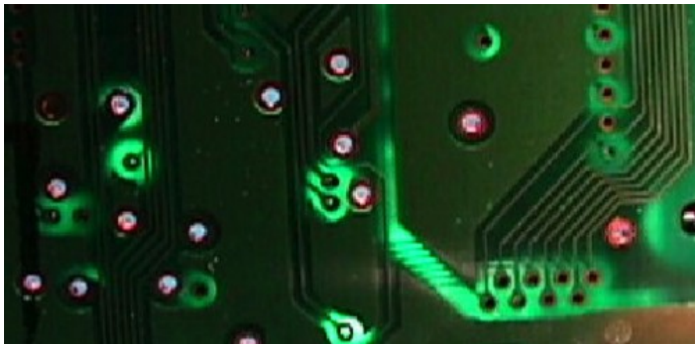
Figure 3. Another Circuit Board Example of Signals Crossing Plane Breaks
