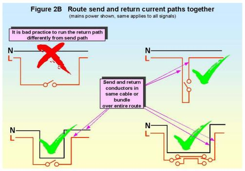
This technique reduces both differential and common-mode the couplings of magnetic and electric fields between the cable and its electromagnetic environment (see Part 1). Although Figure 2B shows a power application this technique is vitally important, for both emissions and immunity reasons, whatever electrical signals or power a cable may be carrying, from weak transducer signals, through high-speed data, to heavy power.
