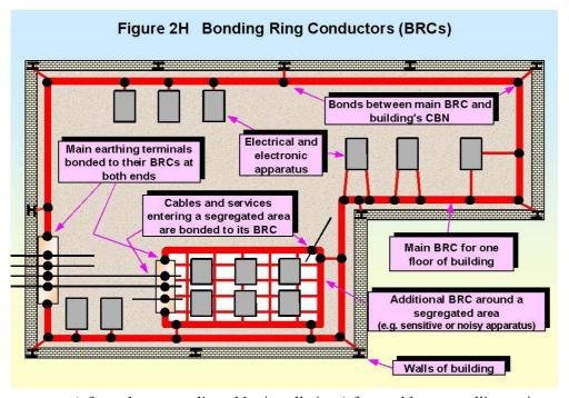
Where it is necessary (often when upgrading older installations) for a cable or metallic service to enter a floor or a zone remotely from its main earthing terminal, it should be bonded (or surge protected and/or filtered) instead to the BRC as it crosses it. But it should be recognised that this is not an ideal situation and the cable or service may need to be re-routed if problems arise.
