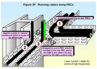
Any part of a properly constructed MESH-CBN may be used as a PEC, and it is best to run a cable over the same type of PEC along its whole length. Of course, PECs must be bonded at each end to the equipment cabinets that the cables enter. They must also be effectively bonded at all joints all along their lengths.
