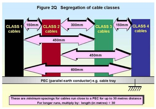
It should be pointed out that there is very little evidence for the cable spacings recommended here. However, we can say with confidence that greater spacings generally give lower coupling (crosstalk) between cables, but the acceptable amounts of coupling will always depend on the types of cables, the installation techniques used, the electronics connected to each end of the cables, and the functional requirements of the application.
