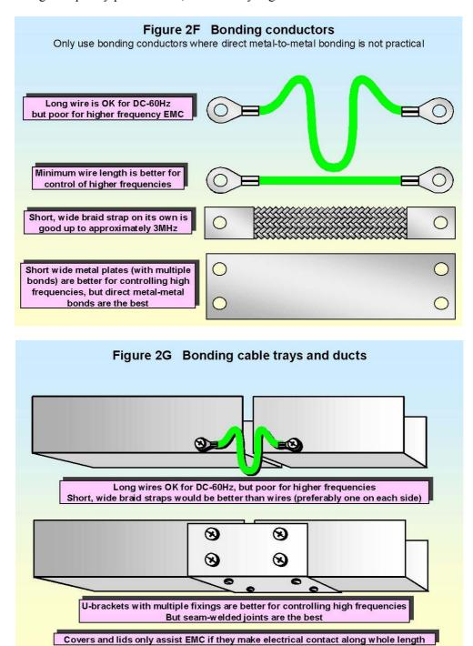
Where high-integrity systems are required to continue functioning despite environmental extremes (especially nuclear and military control rooms) the mesh size of the CBN may need to be reduced so far that metal floors or walls, or even seam-welded metal rooms, become practical options.
