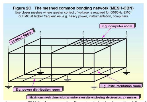
[4]-[10] use the acronym CBN for the common bonding network that is often colloquially referred to as the earthing structure, and they refer to a 3-dimensionally meshed CBN as a MESH-CBN. This is the terminology I shall use throughout the rest of this Part.
