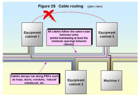
The cable route shown between the different items of equipment in this sketch may be visualised as the stacked cable trays sketched above (for example). Although the cables follow the same route over their common or individual PECs, they should maintain their segregation by class.
