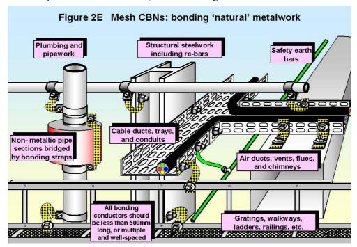
Bonding should ideally be metal-to-metal, and seam welding is best. Short conductors may be used instead with a reduction in high-frequency performance, as shown by Figures 2F and 2G.
