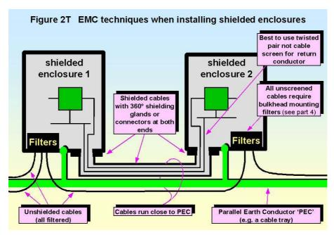
Screened cables should only enter a shielded cabinet through screen-bonding connectors or glands set in the cabinet wall (requiring screen bonding at both ends), and all unscreened cables should only enter through bulkhead mounted filters (or equivalent). All cables between the two cabinets are segregated by class and run in intimate proximity with a PEC that is bonded to both cabinets. This could be a metal cable duct or tray, as described above.
