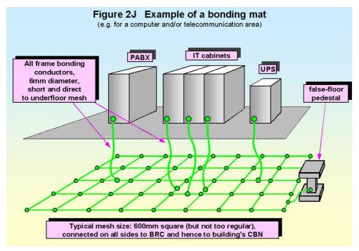
Typically these bonding 'mats' use a mesh of copper wire or lighting tape on a 600mm grid, installed beneath the computer flooring and bonded to the equipment cabinet frames by 6mm CSA cable no longer than 500mm. It is sometimes possible to use the metal support structure for the computer flooring, or metal-covered computer flooring tiles, as a bonding mat. Each bonding mat requires a BRC around its perimeter.
