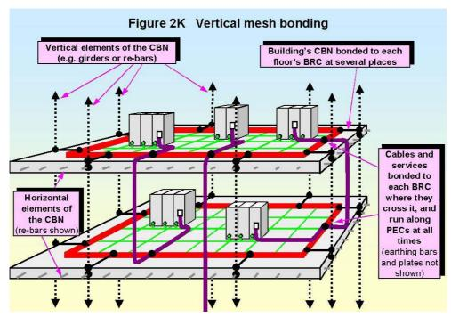
Although each application will differ, a 600mm meshed bonding mat as sketched in Figure 2K ought to be able to achieve the old IBM specification of ground potential differences of no more than 1V over a computer installation. But where better control and/or higher frequencies are required (e.g. where the specification is 15mV and communications use frequencies of up to 30MHz, typical of 100Mbit and Gigabit Ethernets) the grid
