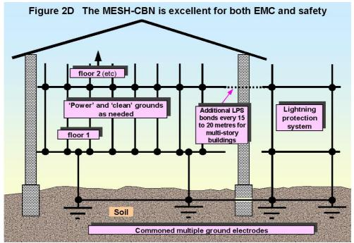
Meshing the CBN helps protect equipment against the damaging effects of lightning surges, and surge protection devices (SPDs) function better when they are connected to a low-impedance CBN. For lightning protection (where most of the energy occurs at frequencies below 10kHz), it is generally recommended that no part of a site should have a CBN whose mesh size exceeds 3 or 4 metres, in any dimension.
