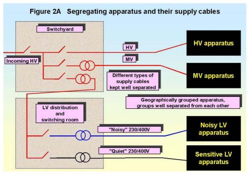
The different classifications of apparatus should be powered via different distribution networks which run separately from each other, and the two (or more) classifications of low voltage equipment should ideally be powered from different distribution transformers. The different classifications of apparatus should be spaced well apart from each other (metres rather than centimetres), and any other cables associated with each type should be routed well away from each other.
