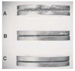
Results of a test comparing lifetime corrosion for three different types of shielding gaskets
