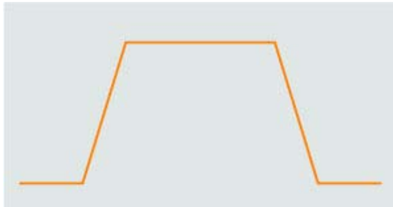
Figure 3: The waveform of an idealized 166-MHz squarewave with 0.6-ns rise and fall times.
