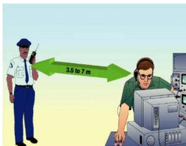
Figure 3. Distance within which a typical private mobile radio handset (walkie-talkie) with 4-W RF power creates an RF field of 3 V/m. Actual distance depends on how nearby metal structures and
