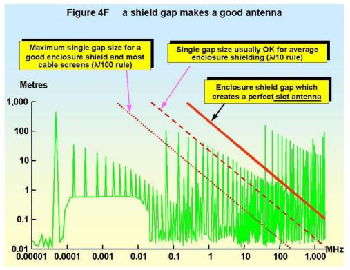
The half-wave resonance of slot antennae (expressed in the above rule of thumb:  $SE = 20\log(\lambda/2d)$ ) is the basis for the solid line in Figure 4F (and for the rule-of-thumb of Figure 4G) using the relationship  $v = f\lambda$  (where v is the speed of light:  $3.10^8$  metres/sec, f is the frequency in Hz, and  $\lambda$  is the wavelength in metres).
