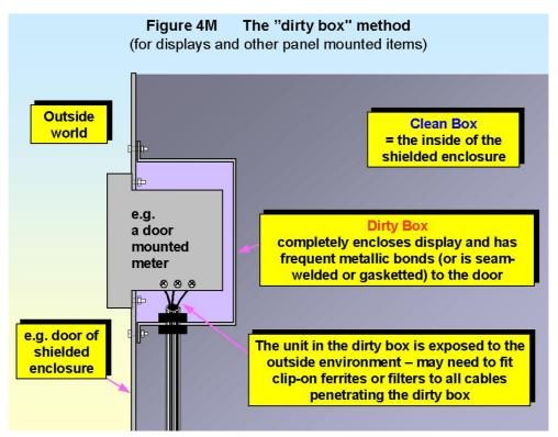
Shielded windows are needed where a display needs shielding by a product's enclosure. Some high-grade CRTs can provide a good shield when the metal frame around the front of their tube is electrically bonded to the front panel all around the aperture. Active matrix LCDs upgrades to products which had used high-grade CRTs have been known to be the cause of more emissions than the CRTs, and some have needed additional shielded windows where the CRTs had not.
