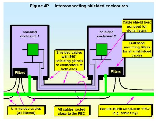
The screens and connectors (or glands) of all screened cables that penetrate a shielded enclosure, and their 360° bonding, are as vital a part of any "Faraday Cage" as the enclosure metalwork itself. The thoughtful assembly and installation of filters for unshielded external cables is also vital to achieve a good SE. These points were made in Parts 2 and 3 of this series, and they are worth making again.
