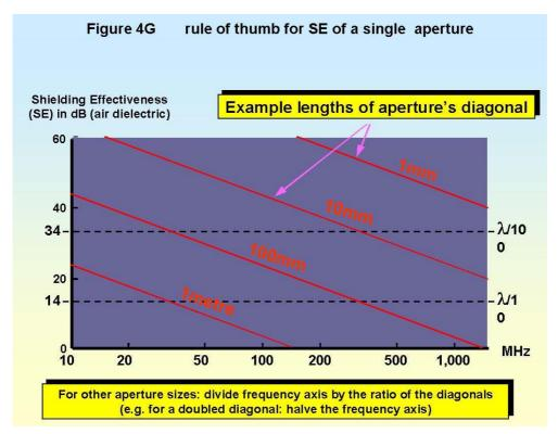
For an SE of 20dB at 1GHz (the present upper limit of testing in most standards) Figure 4G suggests an aperture no larger than around 16mm. For 40dB this would be only 1.6 mm, requiring gaskets to seal apertures and/or the use of the waveguide below cutoff techniques described later.
