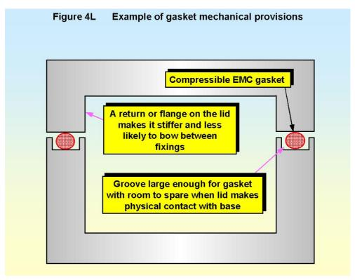
Gasket contact areas must not be painted (unless it is with conductive paint), and the materials used and their preparation and plating must be carefully considered from the point of view of galvanic corrosion.
