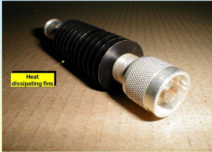
Figure 5F A 20W 50Ω through-line 6dB attenuator
