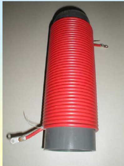
Figure 10 Example of 50 \mu H inductor under construction
