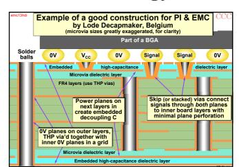
Cost-Effective Use of HDI (microvia) PCB Technology for SI, PI and EMC
