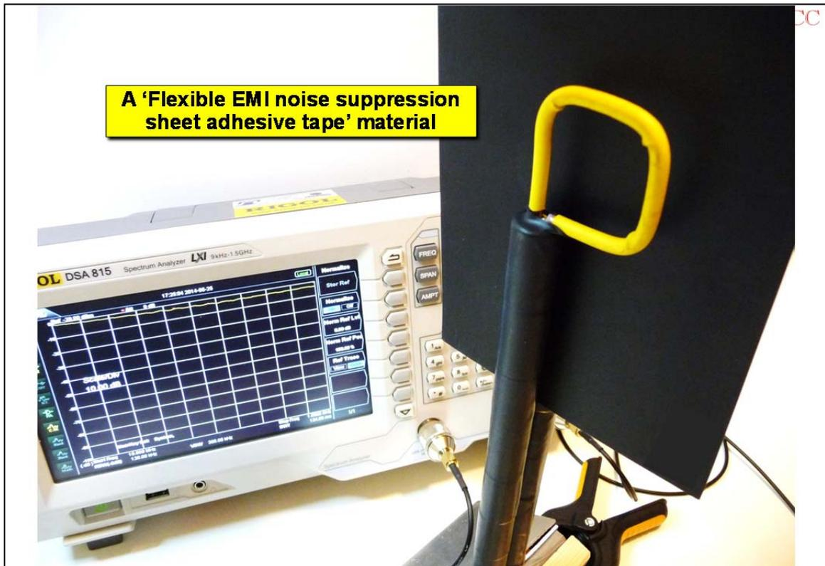
**Figure 75 A 'Flexible EMI noise suppression sheet adhesive tape' material**
