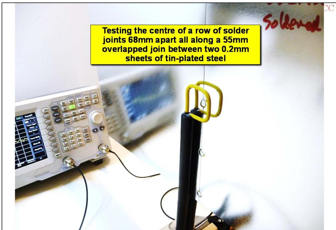
Figure 62 Measuring the 55mm overlapped 0.2mm tin-plated steel
