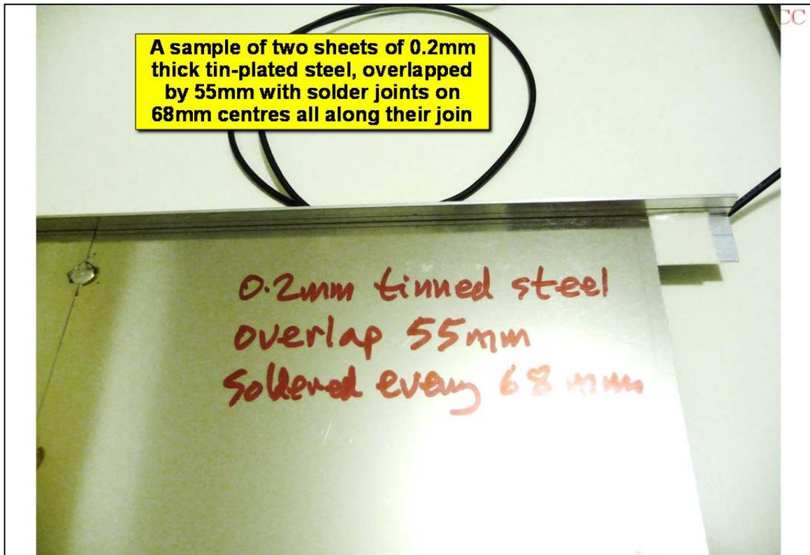
Figure 61 The 55mm overlapped tin-plated steel sheet to be tested
