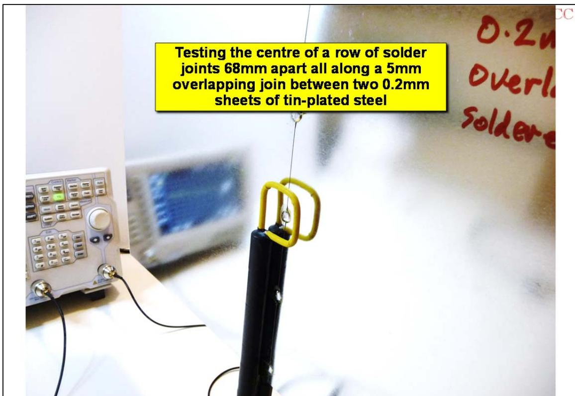
Figure 59 Measuring the 5mm-overlapped 0.2mm tin-plated steel
