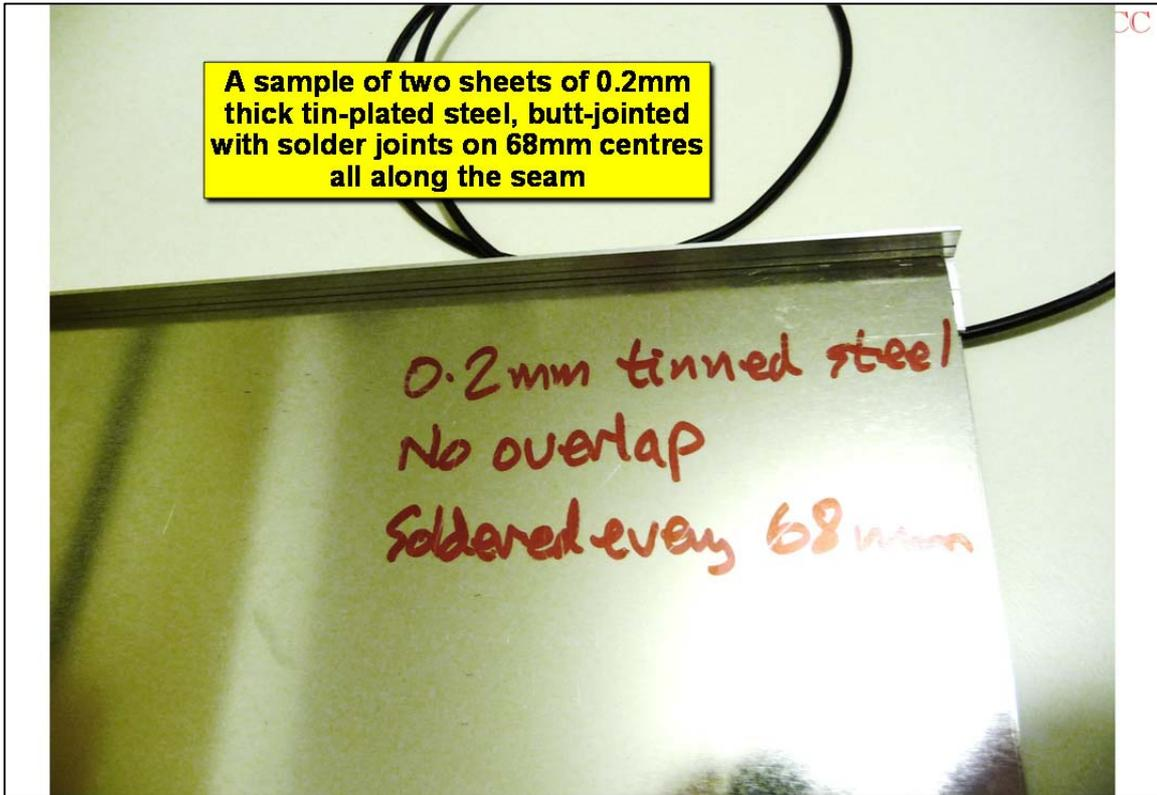
Figure 55 The butt-jointed tin-plated steel sheet to be tested
