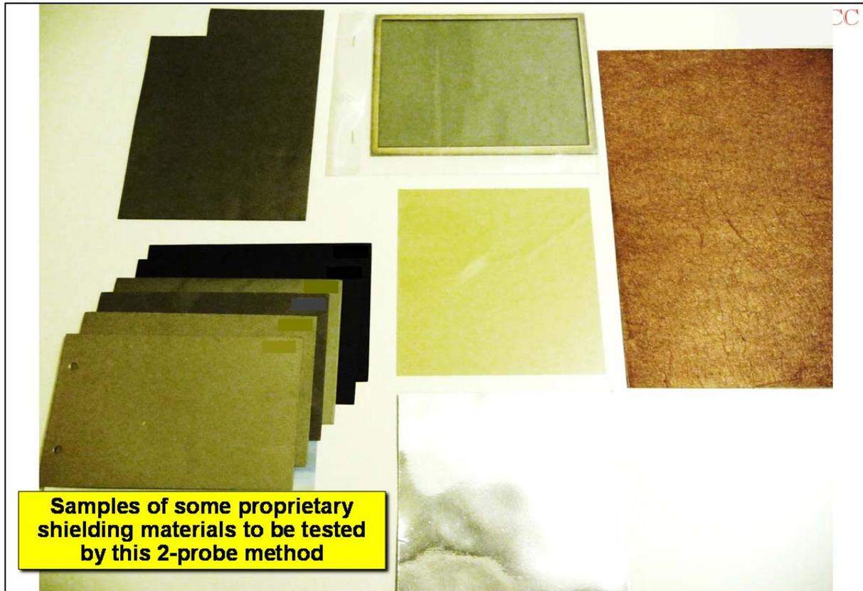
**Figure 64 A range of proprietary shielding materials to be evaluated**
