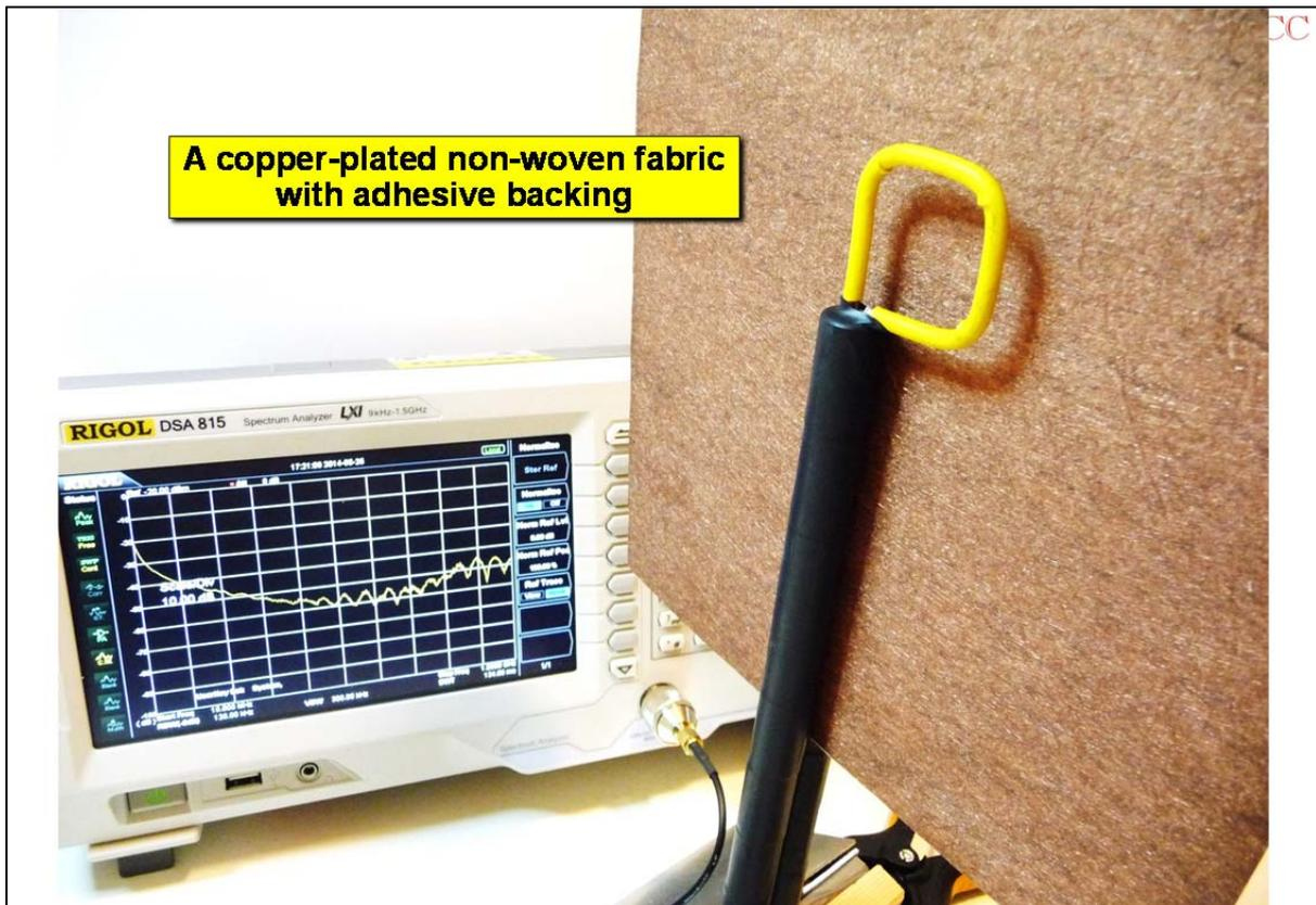
**Figure 65 A copper-plated non-woven fabric with adhesive backing**
