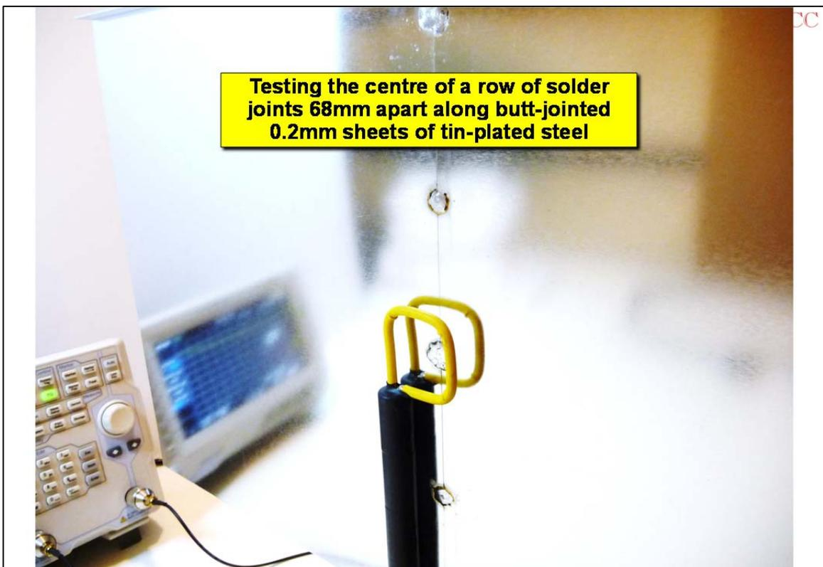
Figure 56 Measuring the butt-jointed 0.2mm tin-plated steel
