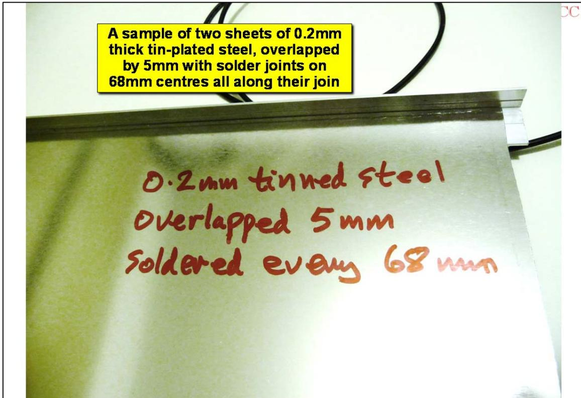
Figure 58 The 5mm overlapped tin-plated steel sheet to be tested
