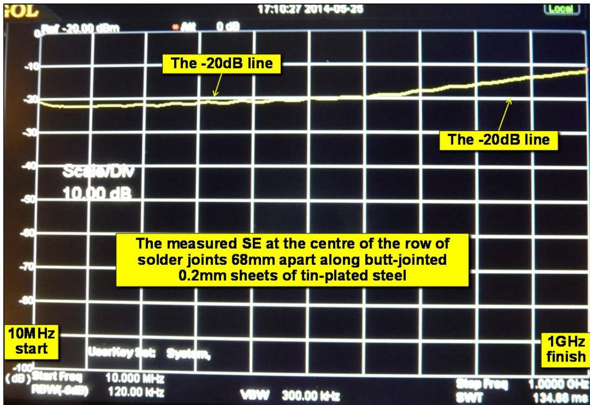
**Figure 57** The analyser's display when measuring the butt-jointed 0.2mm tin-plated steel
