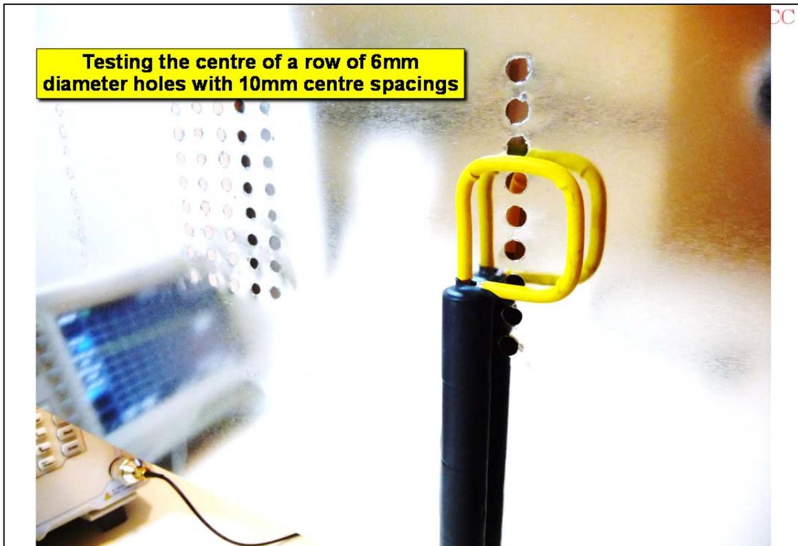
Figure 53 Measuring a line of 6mm holes on 10mm spacing in the 0.2mm tin-plated steel
