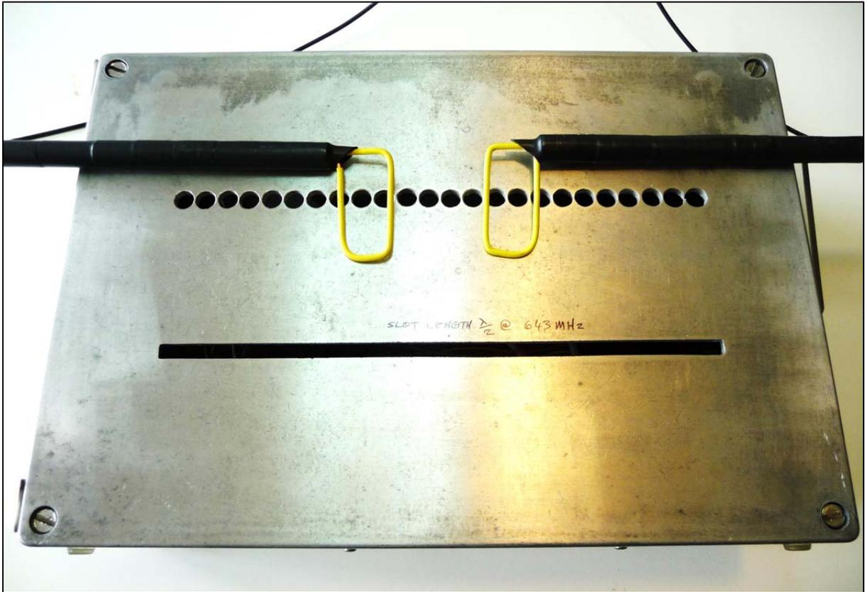
Figure 16 Looking for shield imperfections with two CF probes – the set-up (2)
