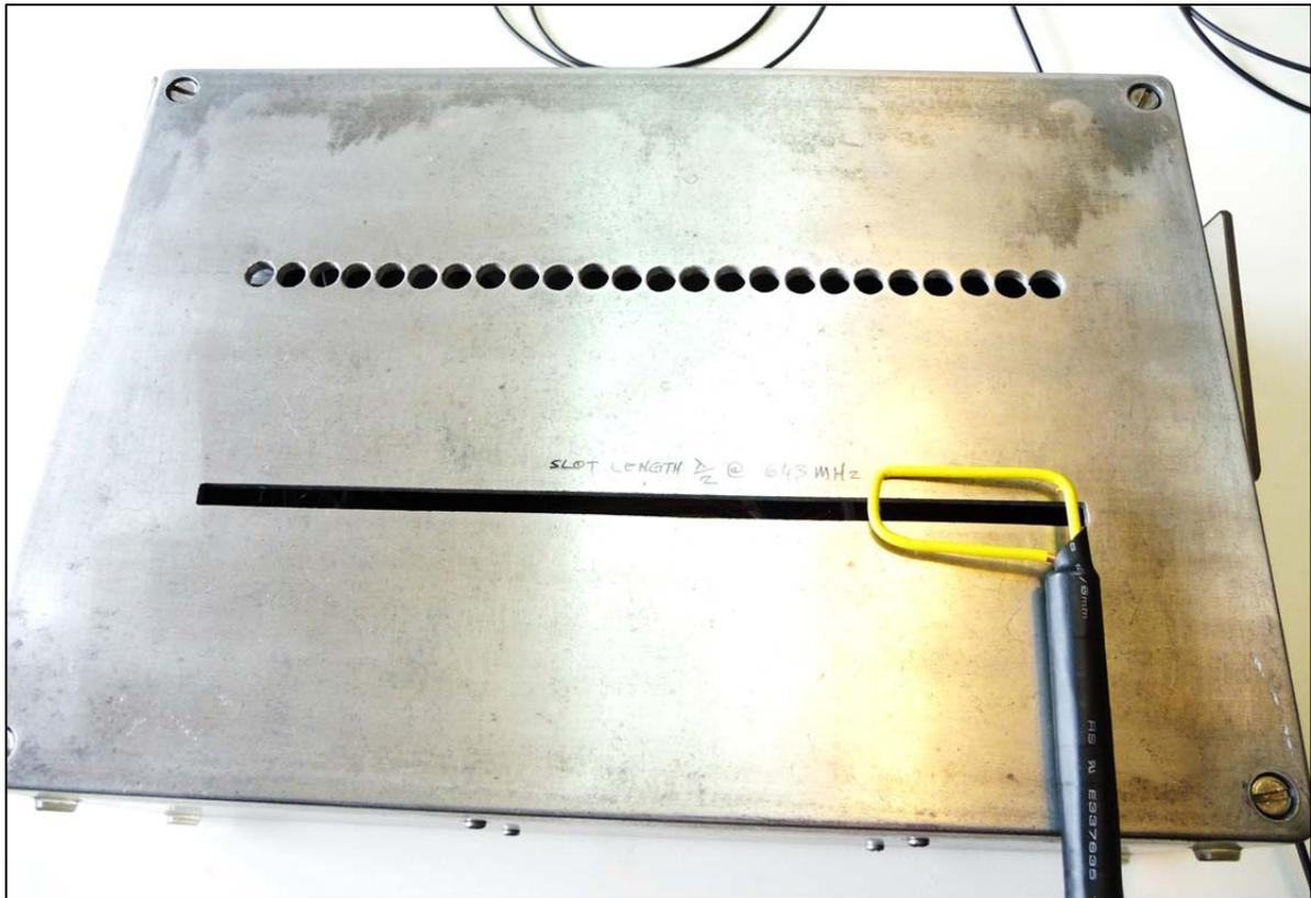
Figure 31 Looking for shielding imperfections with a reflectometer – set-up (8)
