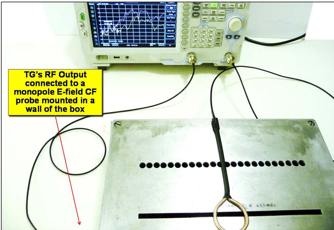
**Figure 37** Looking for shielding imperfections with internal illumination – set-up (11)
