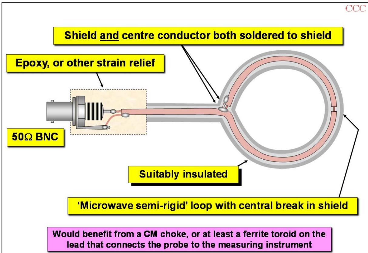
Figure 2 An easier magnetic field close-field probe design (but not so good)
