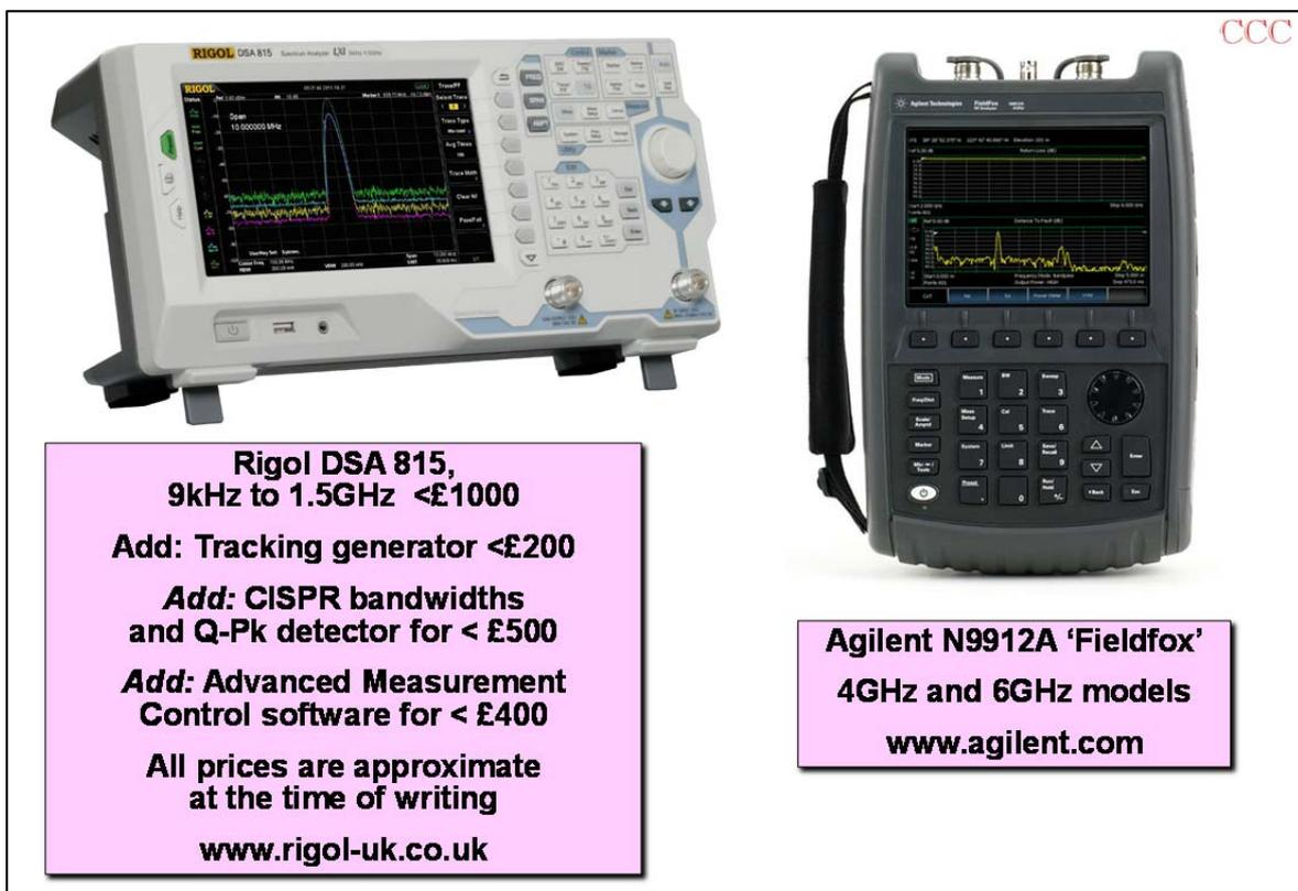
Figure 11 Some more examples of portable and low-cost spectrum analysers
