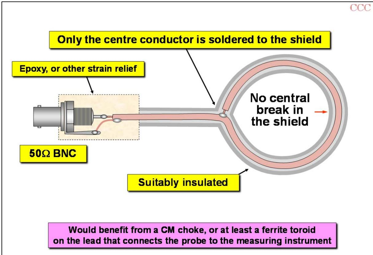
Figure 3 The simplest magnetic close-field probe design (but even less good)
