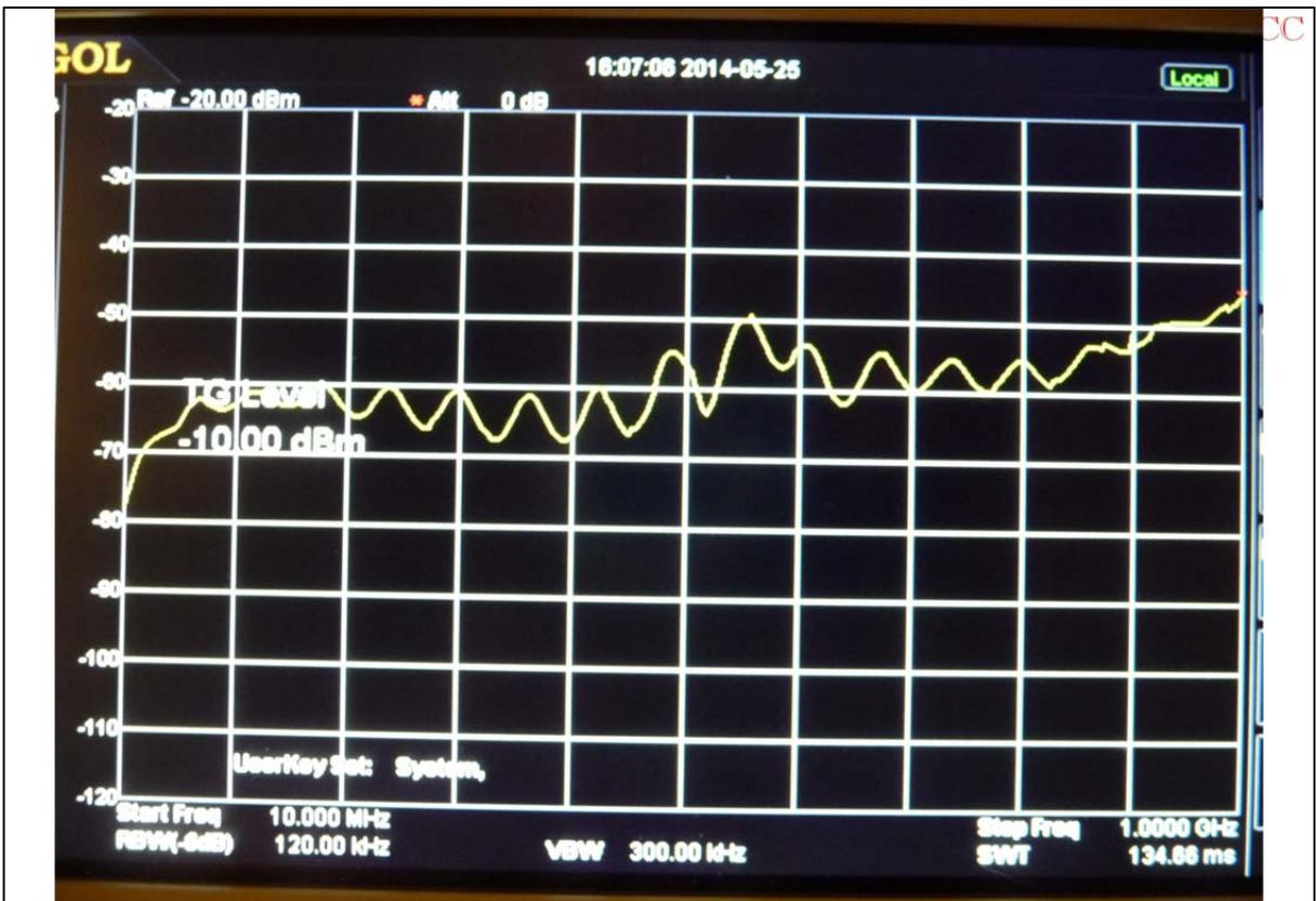
Figure 27 Looking for gasketing imperfections with two CF probes – the display (7)
