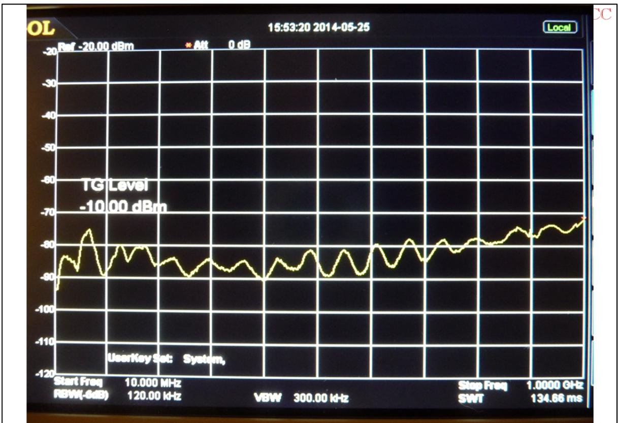
Figure 17 Looking for shield imperfections with two CF probes – the display (2)
