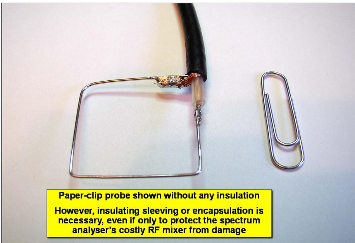
Figure 4 Using a paper clip to make an unshielded close-field probe
