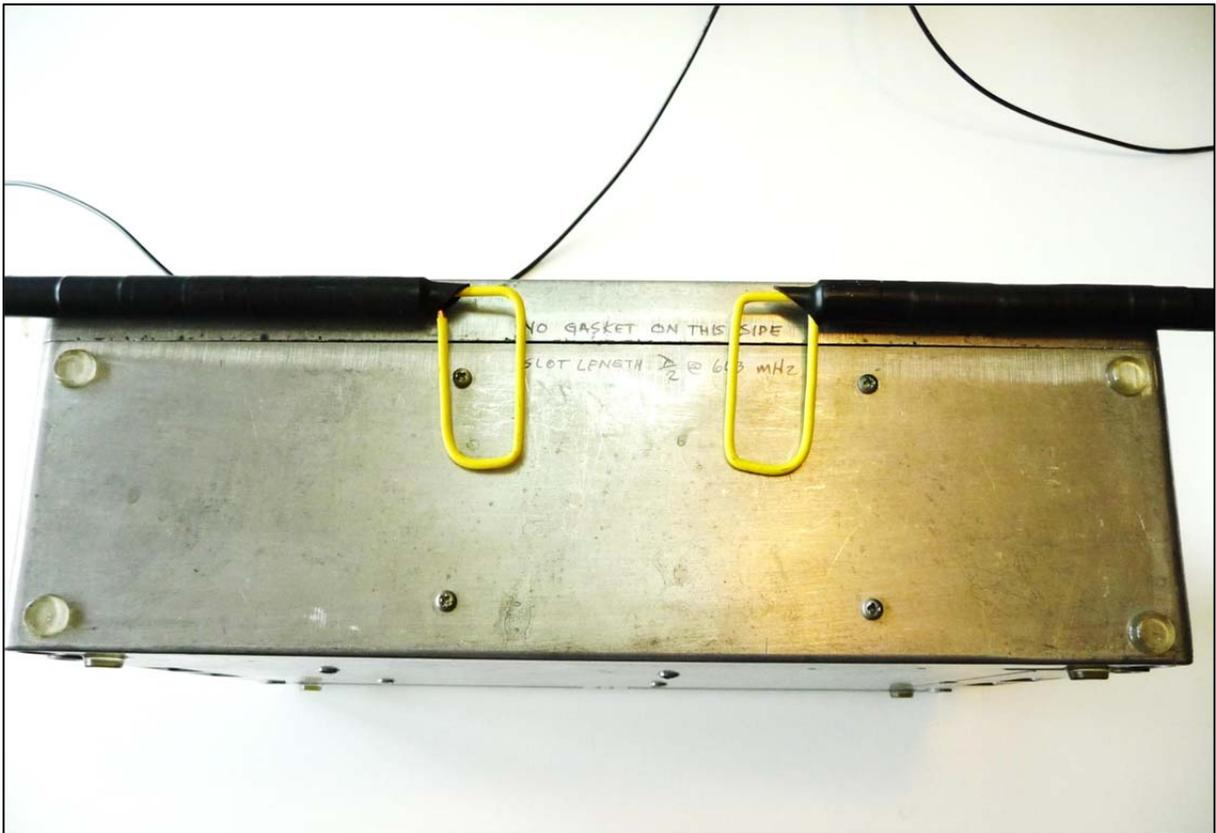
Figure 26 Looking for gasketing imperfections with two CF probes – the set-up (7)
