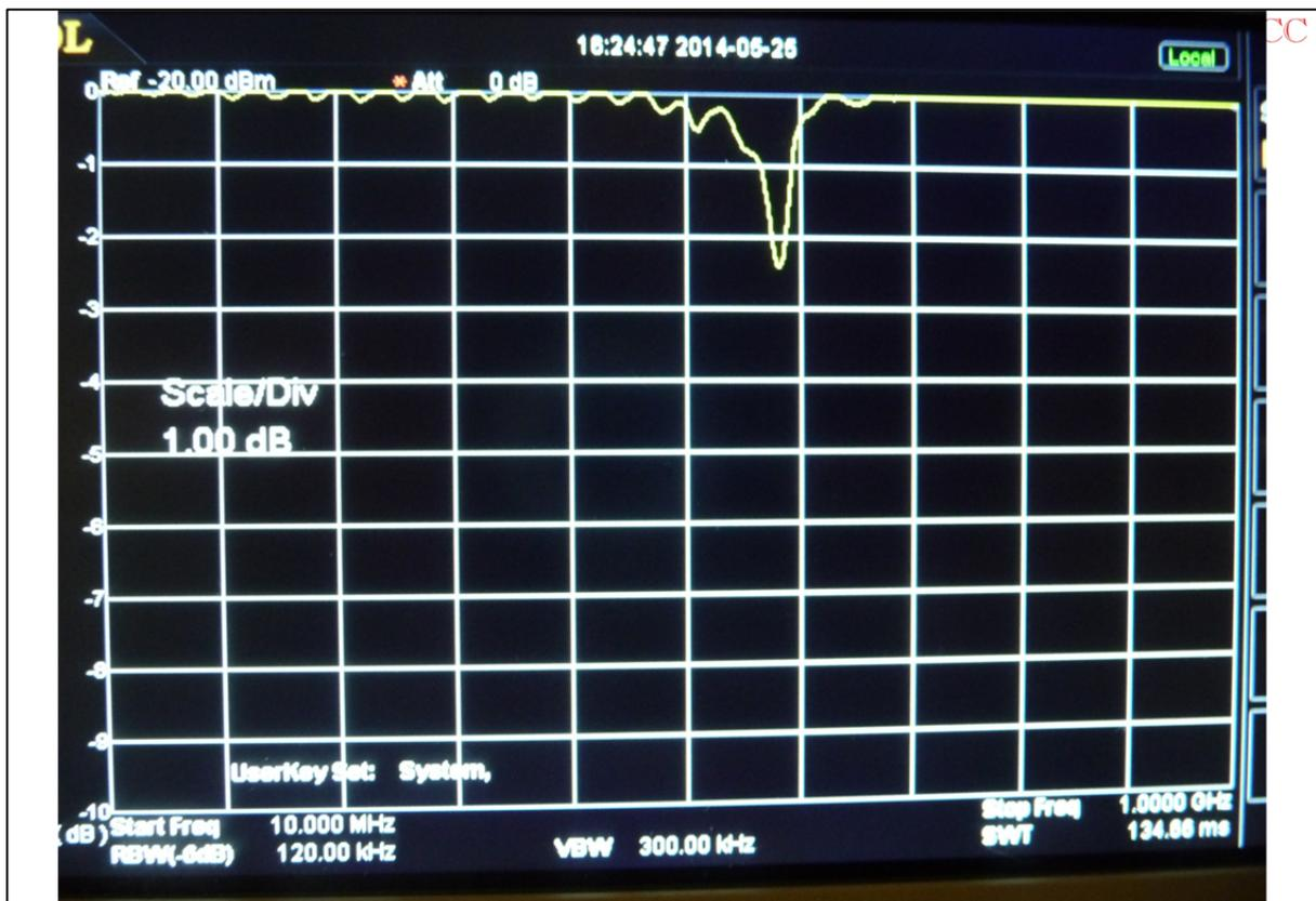
**Figure 34 Looking for shielding imperfections with a reflectometer – the display (9)**
