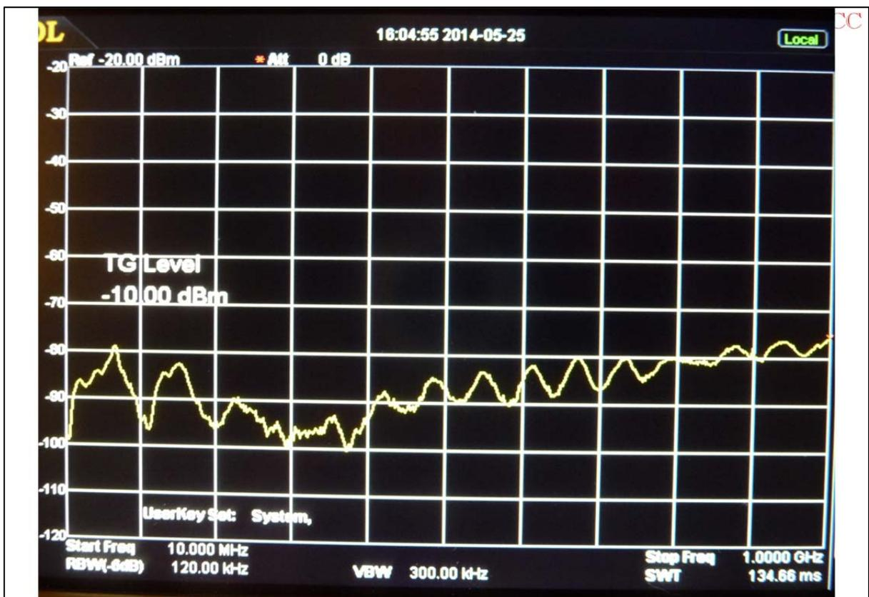
Figure 25 Looking for gasketing imperfections with two CF probes – the display (6)
