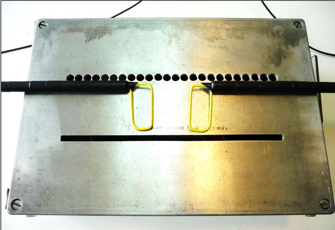
Figure 18 Looking for shield imperfections with two CF probes – the set-up (3)
