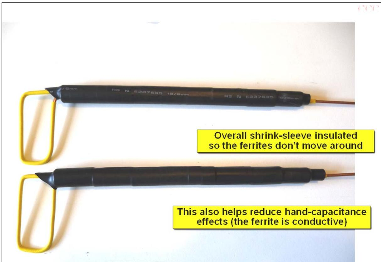
Figure 13 My new RG405 probes when finally assembled
