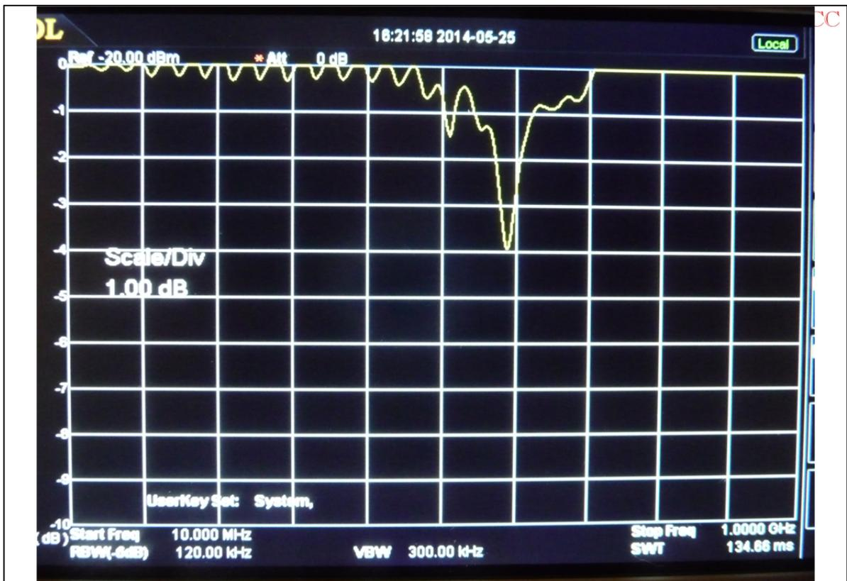
Figure 32 Looking for shielding imperfections with a reflectometer – the display (8)
