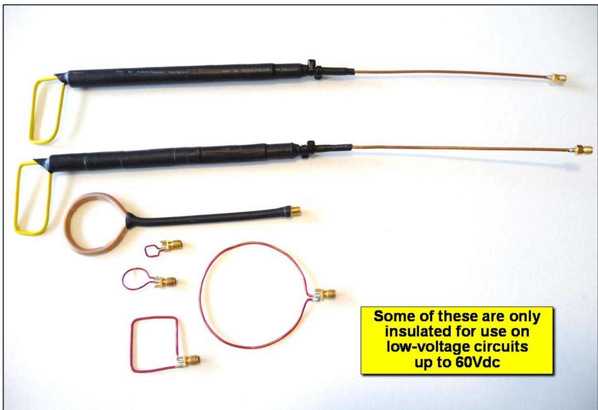
**Figure 5** The range of close-field probes that I use (at the time of writing)
