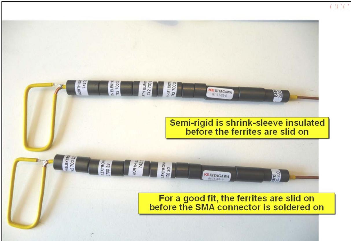
Figure 12 A view of my new probes during assembly
