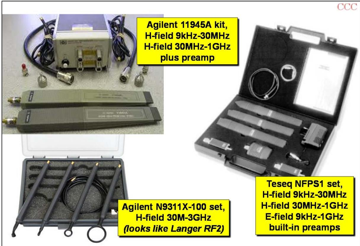
Figure 8 Hewlett-Packard's venerable close-field probes, and currently available ones from Agilent (soon to be renamed Keysight Technologies) and Teseq (which used to be Chase EMC)
