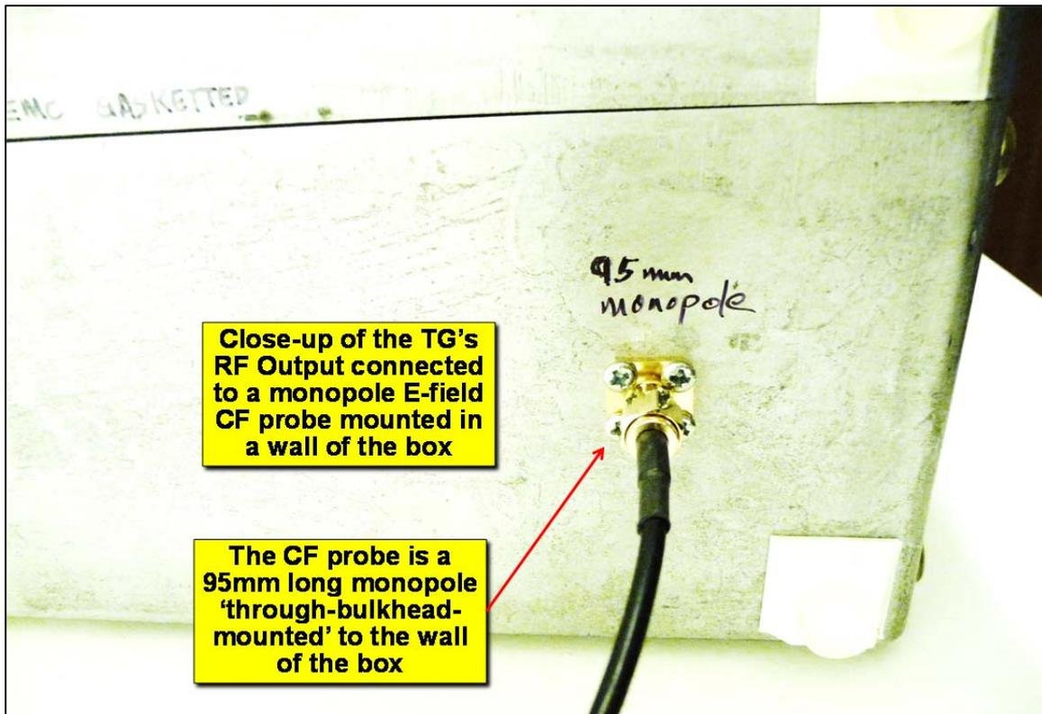
Figure 36 Looking for shielding imperfections with internal illumination – the internal CF probe
