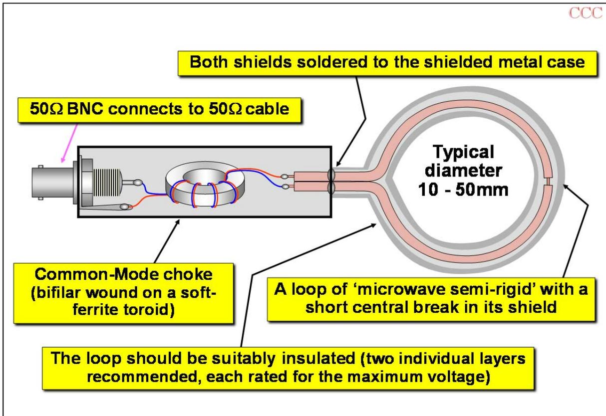
Figure 1 The construction of a good-quality close-field magnetic probe
