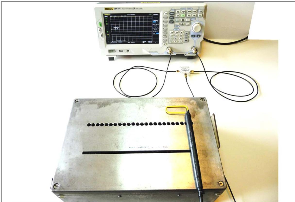
Figure 28 Looking for shielding imperfections with a reflectometer – normalising
