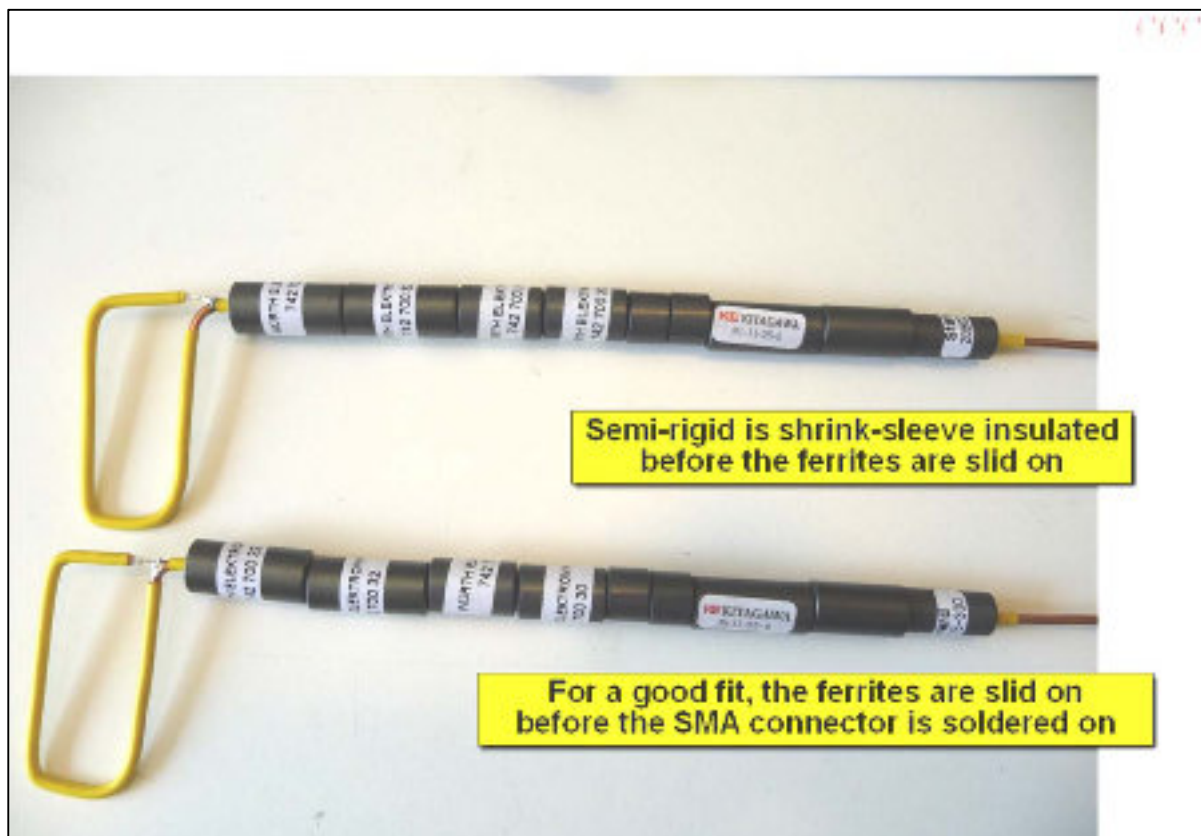
Figure 12 A view of my new probes during assembly
