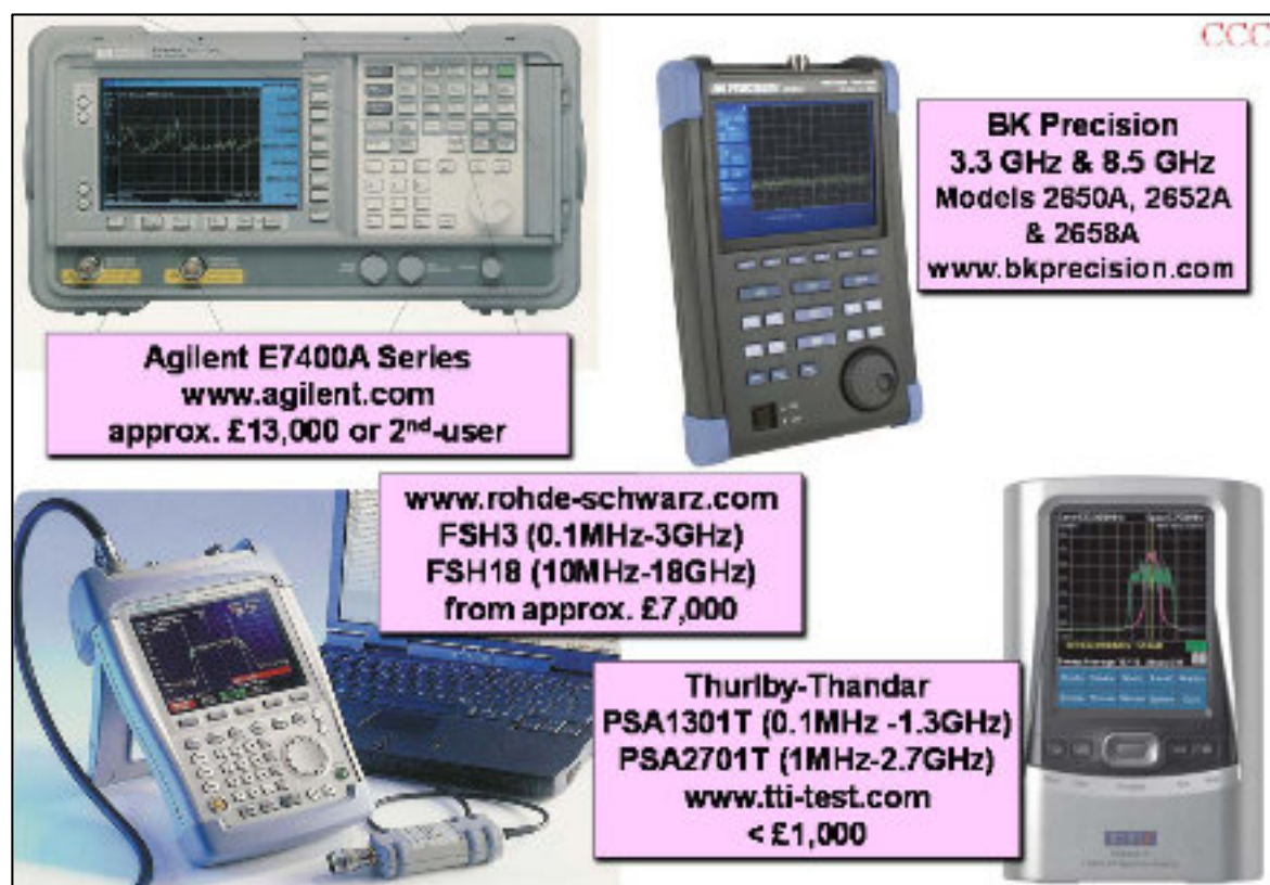
Figure 10 Examples of portable spectrum analysers, including some very low-cost ones
