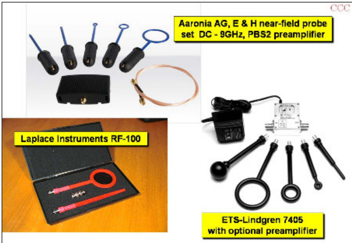
Figure 6 Examples of close-field probes from Aariona, Laplace Instruments and ETS-Lindgren
