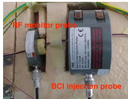
Figure 1 BCI injection probe and RF monitor probe set-up for BCI test
