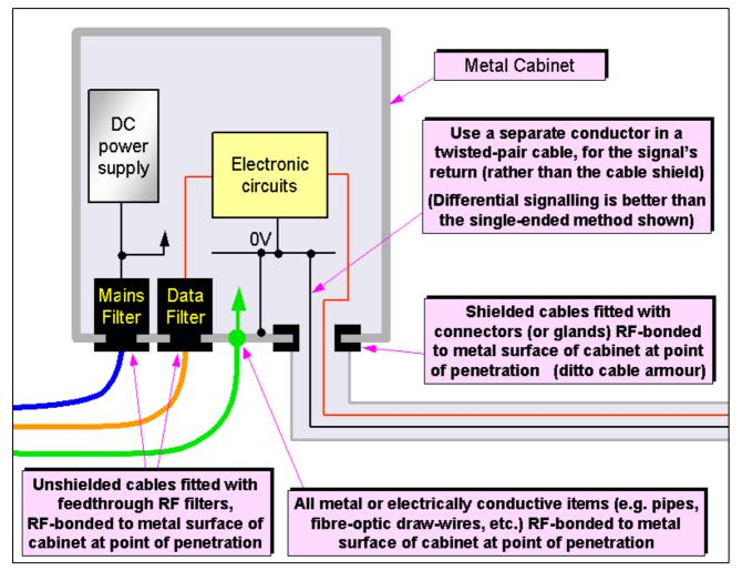
RF-bonding techniques suitable for mains filters were covered briefly by this column in the November 2007 Edition, which also covered how to choose appropriate mains filters in the first place. Filters for signal, data and control cables should be RF-bonded similarly – but the method described for choosing mains filters does not apply because manufacturers only provide  $50\Omega$  data for signal/data filters.
