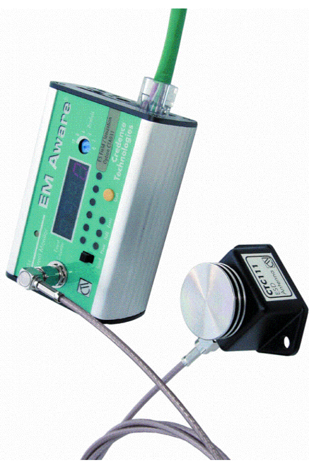
Example of an ESD event detector (courtesy of Credence Technologies, Inc.)
