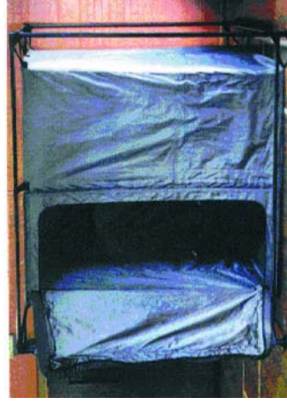
An example of a low-cost shielded tent
